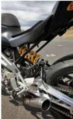
ABOVE: The stock 2002 Ducati 900SS motor is fitted with a Power Commander to optimise the modified shorty exhaust
