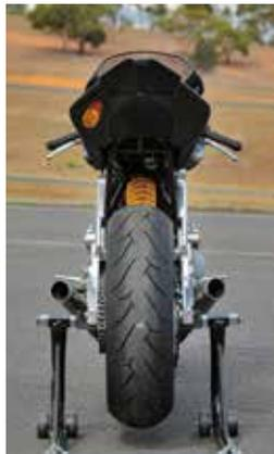
ABOVE: The rear shock is operated by the machined billet-aluminium swingarm pivoting in the Ducati engine's crankcases, via a direct-action cantilever
