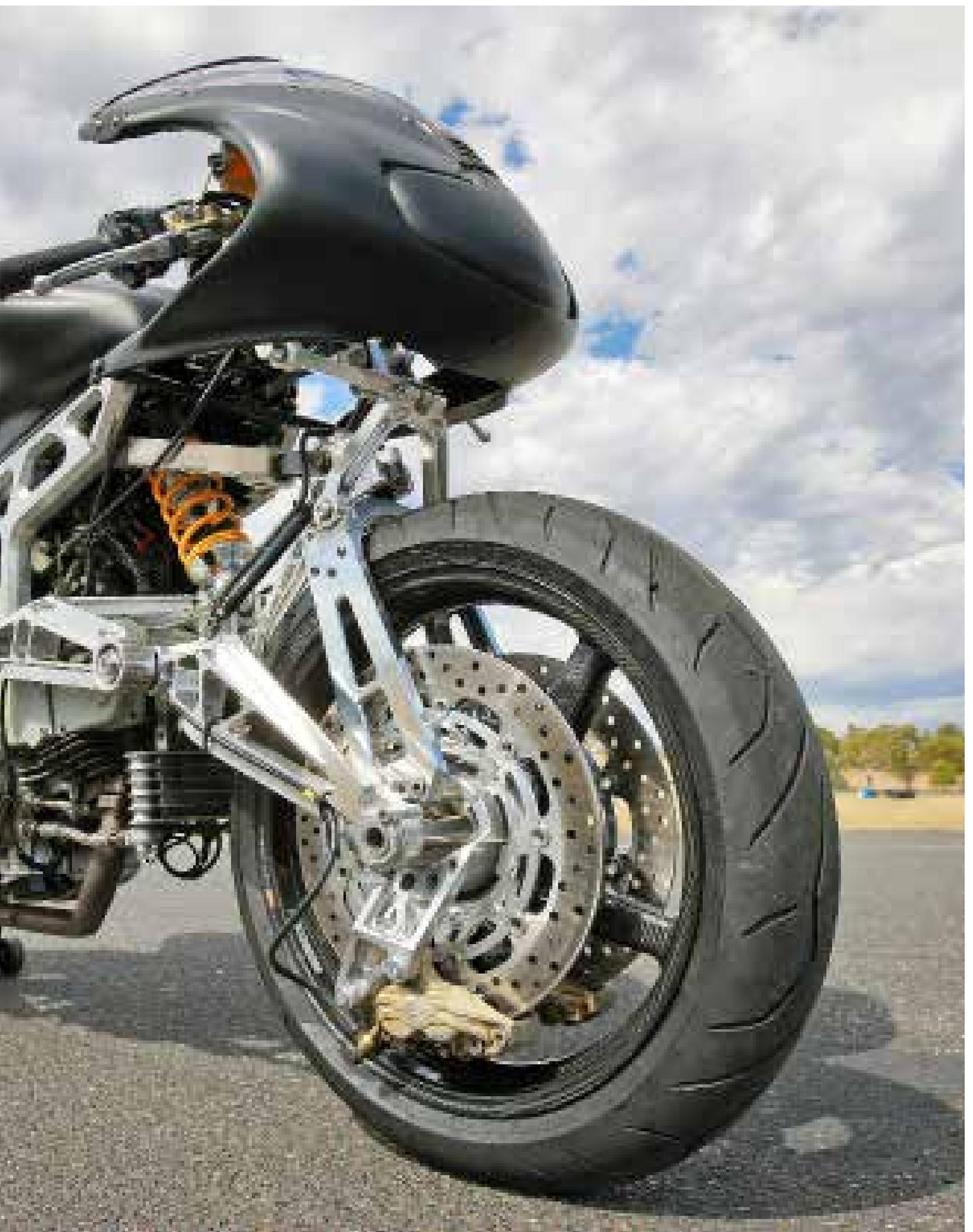
2002 Ducati 900SS engine in a radical chassis as the platform to develop their unique front-end suspension and separate steering system, for what they hope will be eventual worldwide sale. And since I may immodestly claim to have extensive experience of both riding and racing motorcycles with alternative front-end designs, they invited me to come and sample the result.
