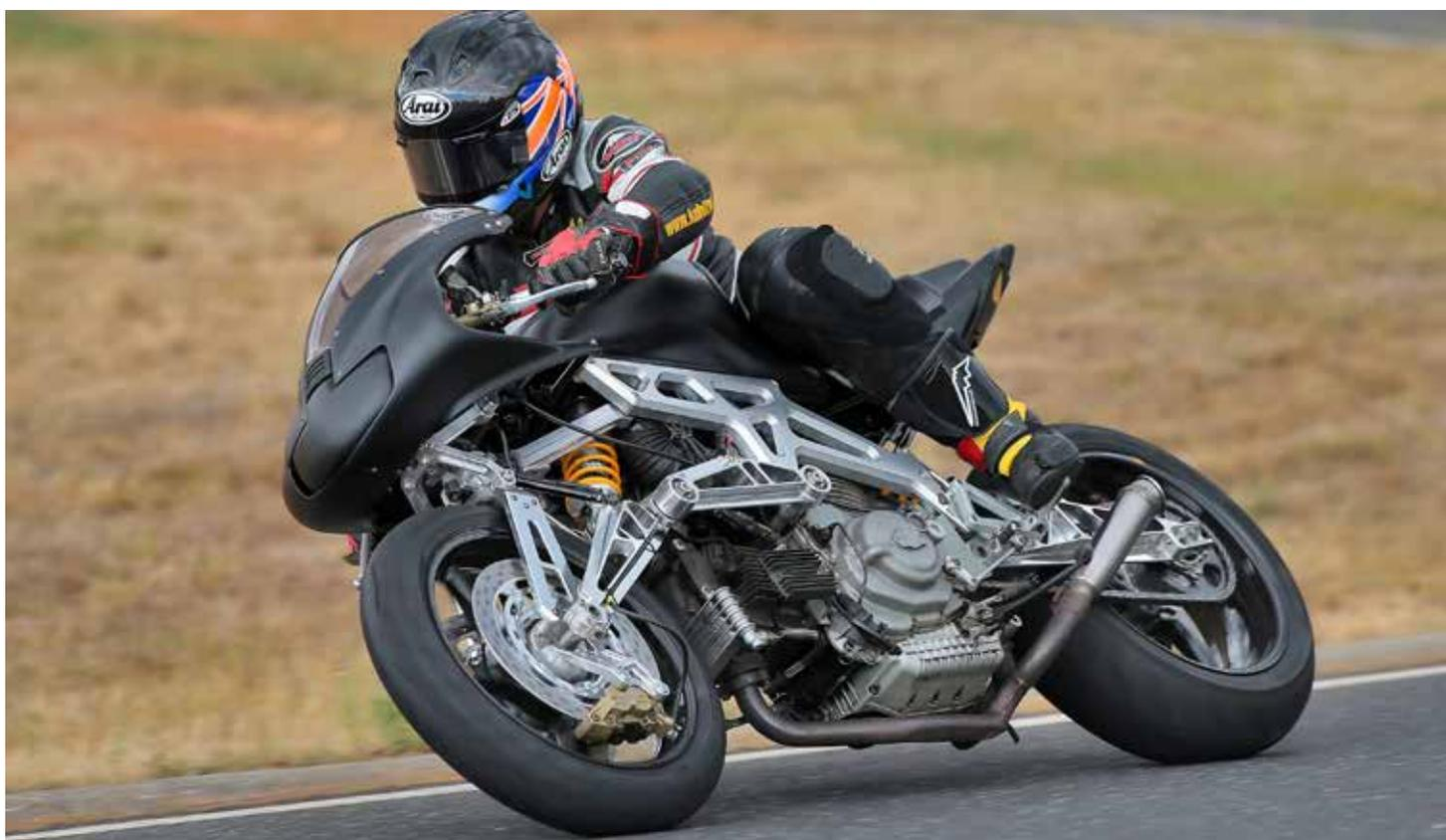
to lift the front wheel over the first step. Even though there was no steering damper, it would only flap the front wheel once very quickly, before resuming normal service. And best of all it was very stable under hard braking from high speed, even trailbraking into the off-camber right at the end of the straight, with not a trace of the shimmy it had suffered from previously.
